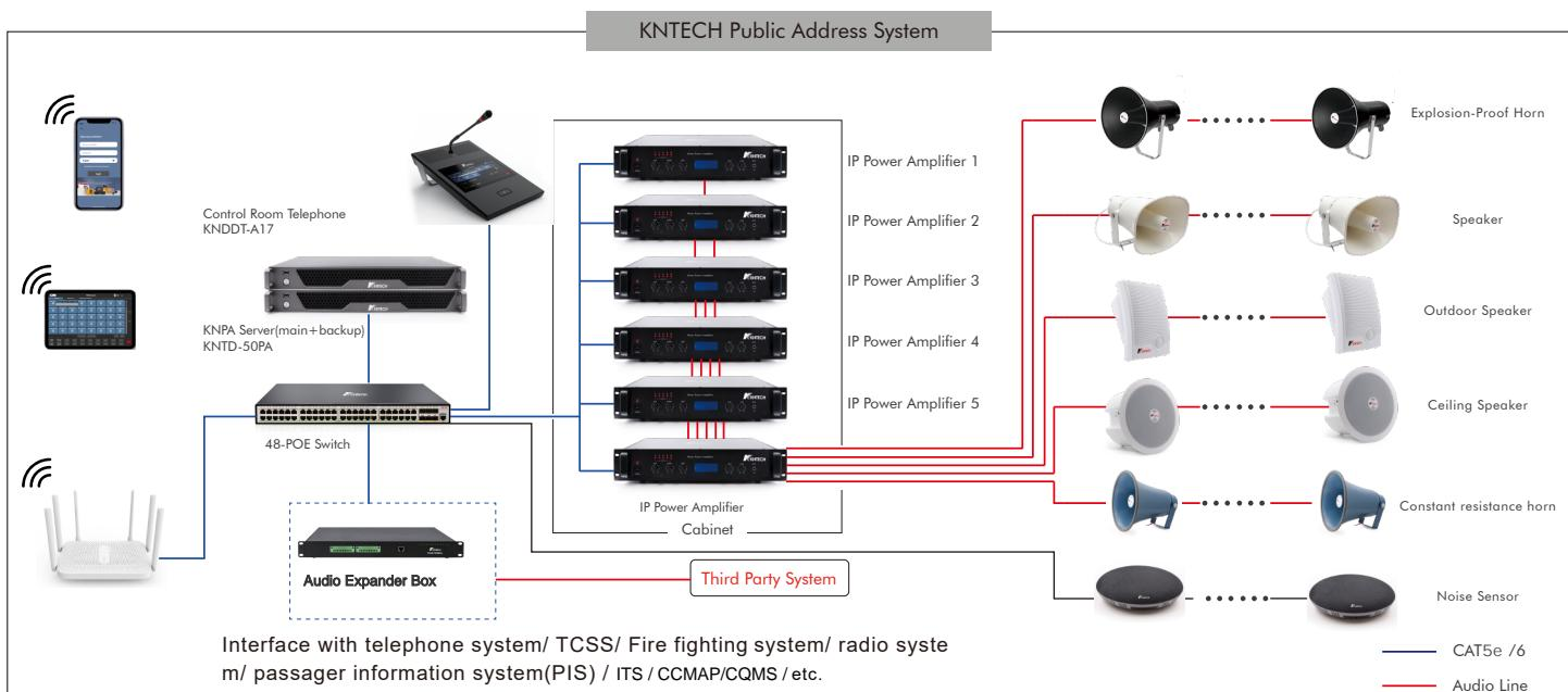
The core of the PA system is the KNPA-50 server. The mobile phone installs PA-App to carry on the broadcast operation to the broadcast system terminal. The whole system consists of many types of broadcast terminals, users can choose a variety of broadcast terminals based on the actual situation.
